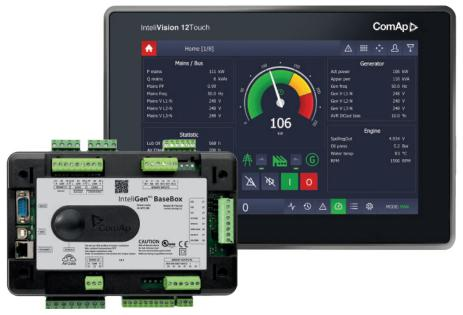
ComAp's Power Management System provides fully automatic operation of the generators including load dependent start/stop, power band control, running hours' equalization, automatic synchronization and load-sharing. ComAp's Power Management System offers a reliable, continuous and effective solution for power generation which can be also used for variable speed generators or shaft generators.
